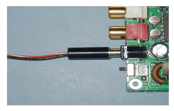
Next connect the Video cable for the TFTOPPER to the Media Board as shown below.
