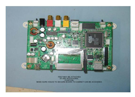
Next locate the power connector on the Media board and the 2.5MM Connector on the Power "Y" Adaptor.
